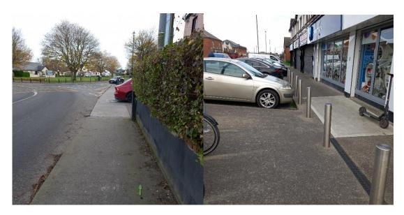
Perdendicular parking with inadequate widths for car overhang can cause damage to existing posts and signs.
