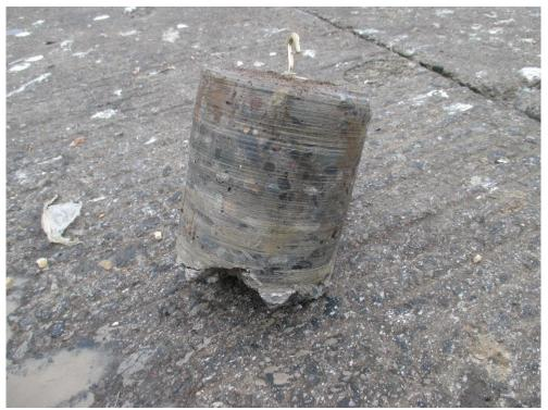
Fig 4.1.4 - Typical Core Section Removed
