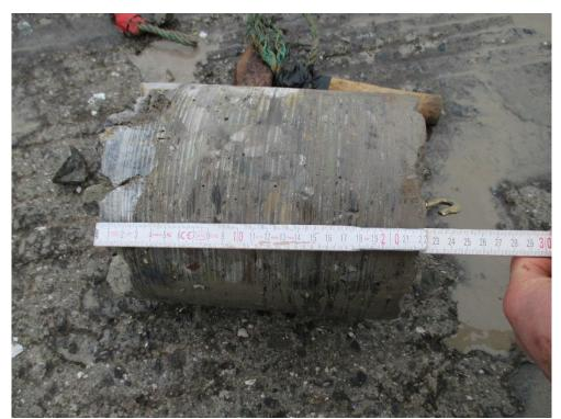
Fig 4.1.3 - Concrete Slab Thickness
