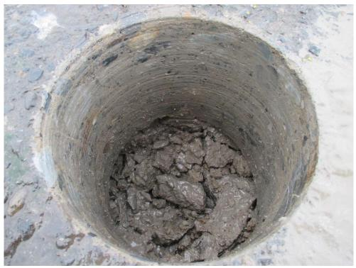
Fig 4.2.7 - Fill material within hole No. 4
