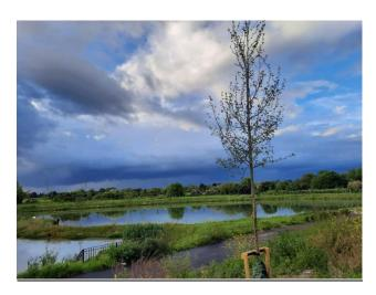
The GDSDS has outlined SuDS as a sustainable way to manage surface water as we prepare to meet the challenges of climate change. This example of Millers Glen in Swords, shows an example of surface water being held onsite, providing treatment via appropriate planting, and then discharging at greenfield runoff rate. This is a move away from the traditional method of collecting all surface water via piped systems which can often no longer manage the intense rainfall's being experienced.
