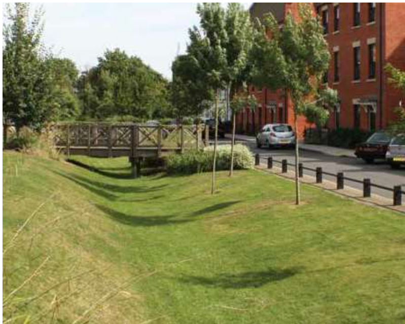
Image 5.10 - Example Roadside Swale (CIRIA C753)
