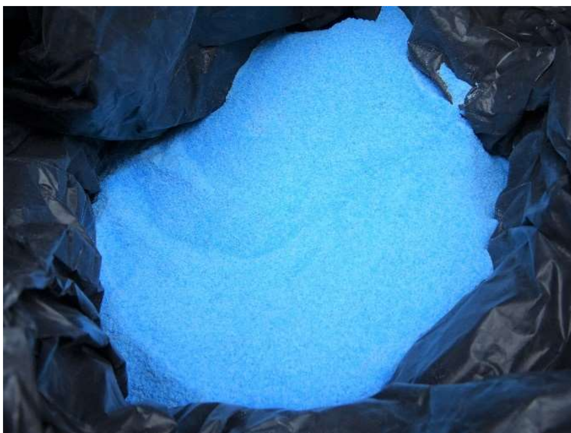
Copper sulphate or bluestone crystals ready for use by the thatcher Alan Grimes
