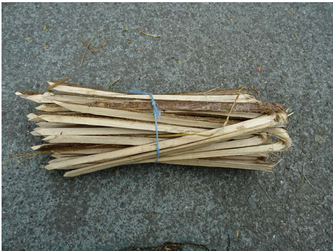
A bundle of hairpin scollops ready for use by thatcher Alan Grimes
