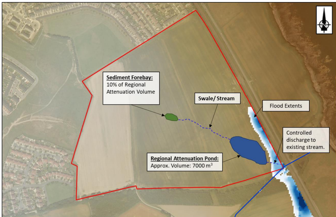
Figure 25: Regional Attenuation – Approximate Location & Sizing
