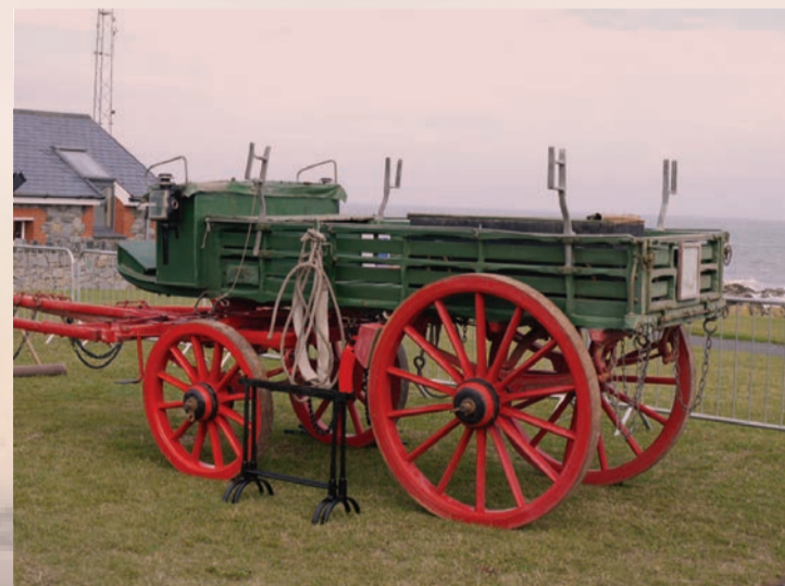
Skerries Rocket Cart Courtesy of the Irish Coast Guard Service, Skerries The Rocket Cart is a lifesaving apparatus. A rocket was used to shoot a light rope onto a ship in distress. This rope was then used to pull heavier ropes and equipment onto the ship. The Rocket Cart contained a supply of lifesaving equipment and was usually horse-drawn. The Skerries Rocket Cart is currently on loan to Fingal County Council.
