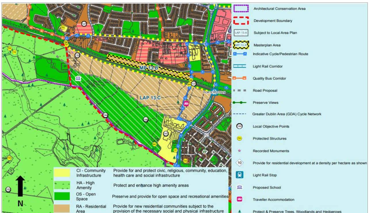
Figure 3.1: Extract from the Development Plan Zoning Map Sheet 13 showing the area of Kellystown LAP (LAP 13.C)
