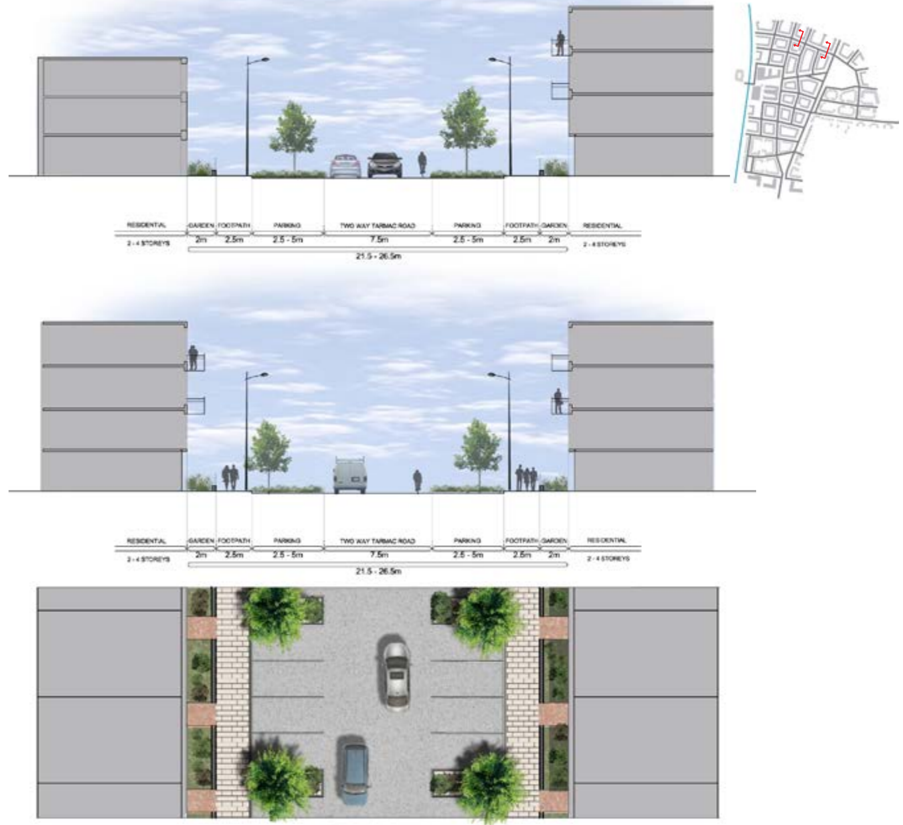
Figure 5.10 Section through Stapolin Way
