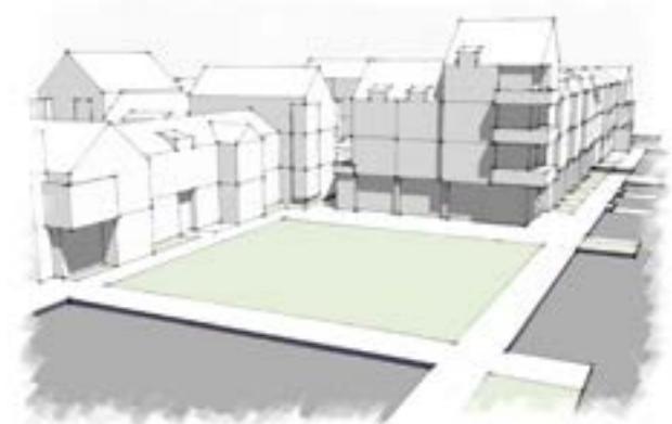
Figure 5.38 The design of the dwellings surrounding pocket parks will require careful consideration in order that they can play the dual role of providing natural surveillance of these park areas while also ensuring that the occupants of the dwellings are afforded a high degree of privacy.
