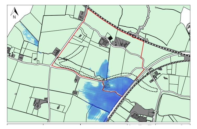
Figure 2.7a Predicted flood extent for 100 and 1000 year flows with proposed road in place a: 100 year flood extent with proposed road in place
