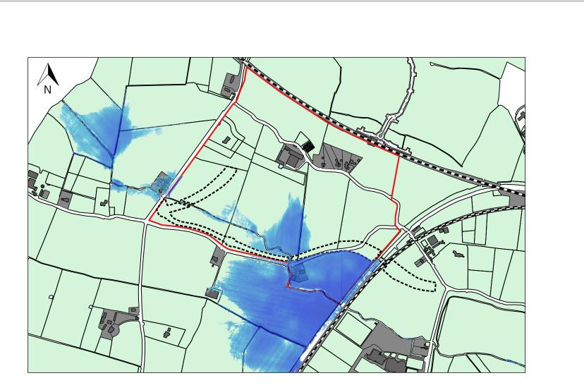
Figure 2.7b Predicted flood extent for 100 and 1000 year flows with proposed road in place b: 1000 year flood extent with proposed road in place
