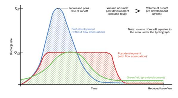
Figure 3.1 Example of a runoff hydrograph for a storm event (Source: www.ciria.org)
