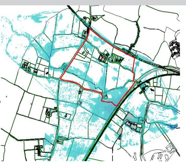
The model is based on the Flood Modeller software package. A regular grid size of 5m was used with a time step of 1 second and global roughness (Manning's n) value of 0.07.
