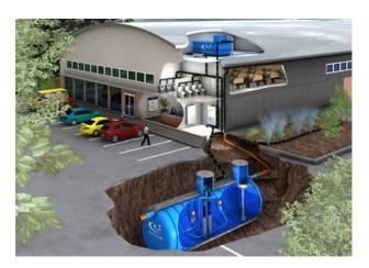
Photo 3.6.2 Rainwater Harvesting Schematic (Source: www.techpreviiew.org)
