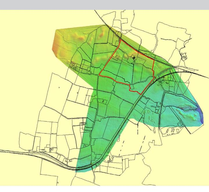
Figure 2.5 LiDAR coverage (shaded area) and development site boundary (red)
