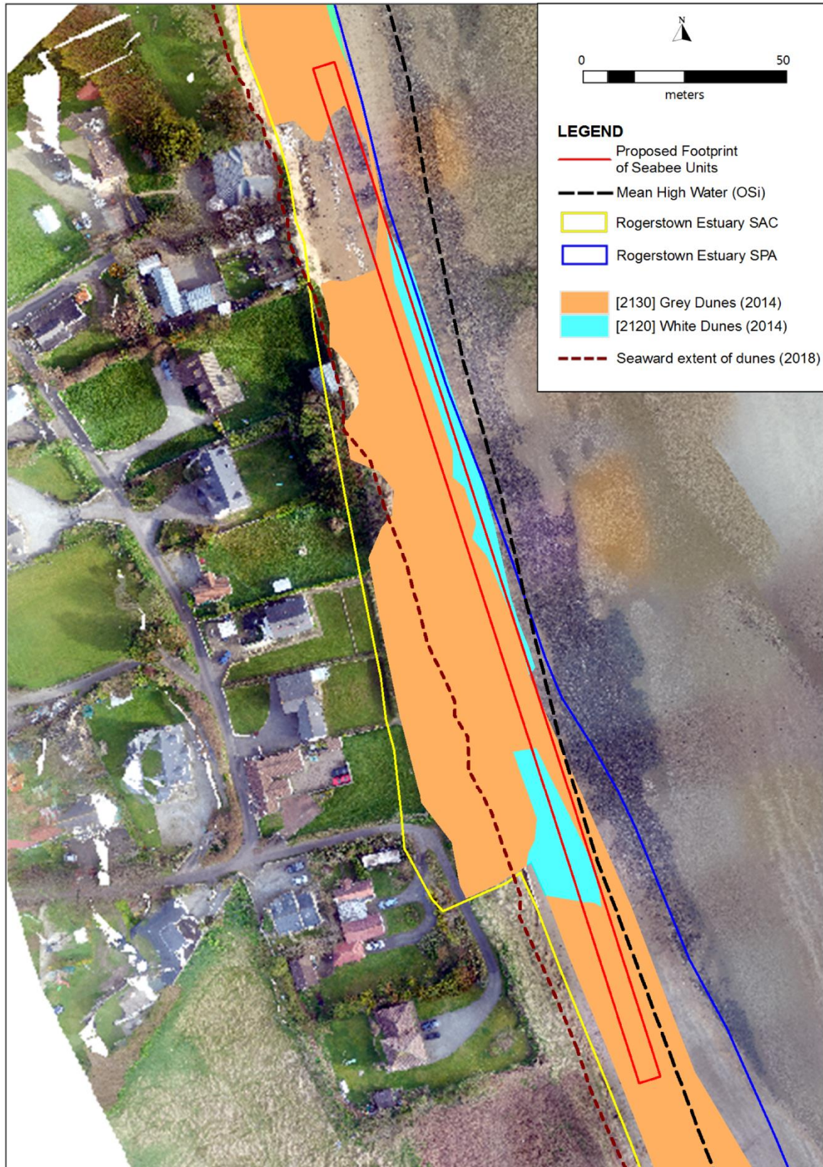
Figure 4.21: Former Annex I sand dune habitats at the location of the proposed Seabee units
