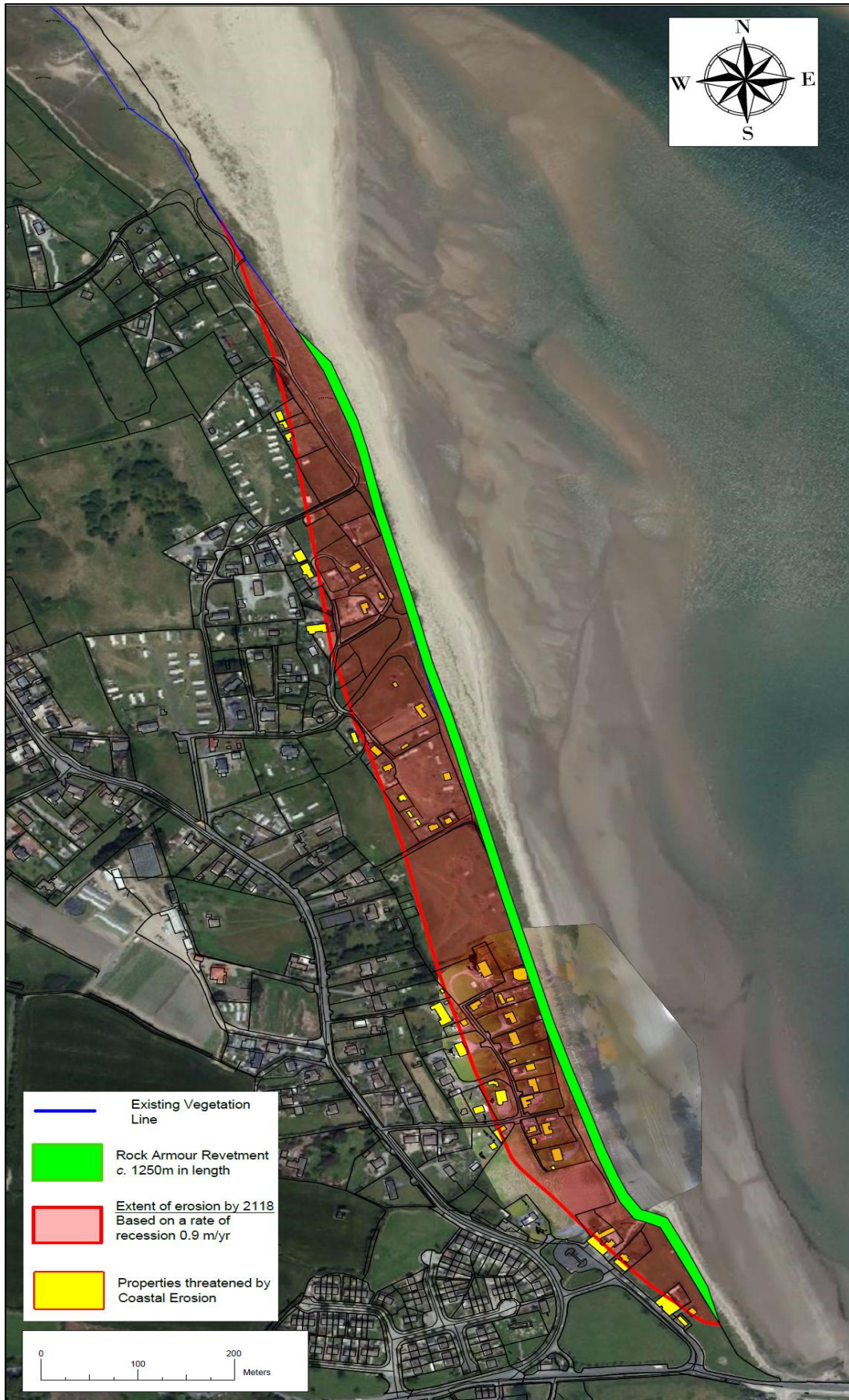
Figure 6.1: Layout and extent of a typical revetment structure (shown in green) that could be constructed along the Burrow to protect against erosion.
