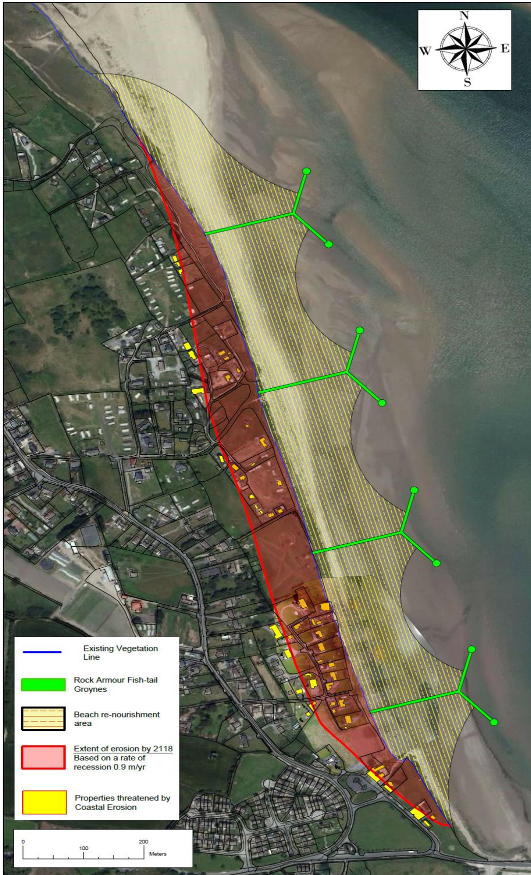
Figure 6.2: Layout and extent of a series of fish-tail groynes and beach renourishment areas that could be implemented along the Burrow to protect against erosion.
