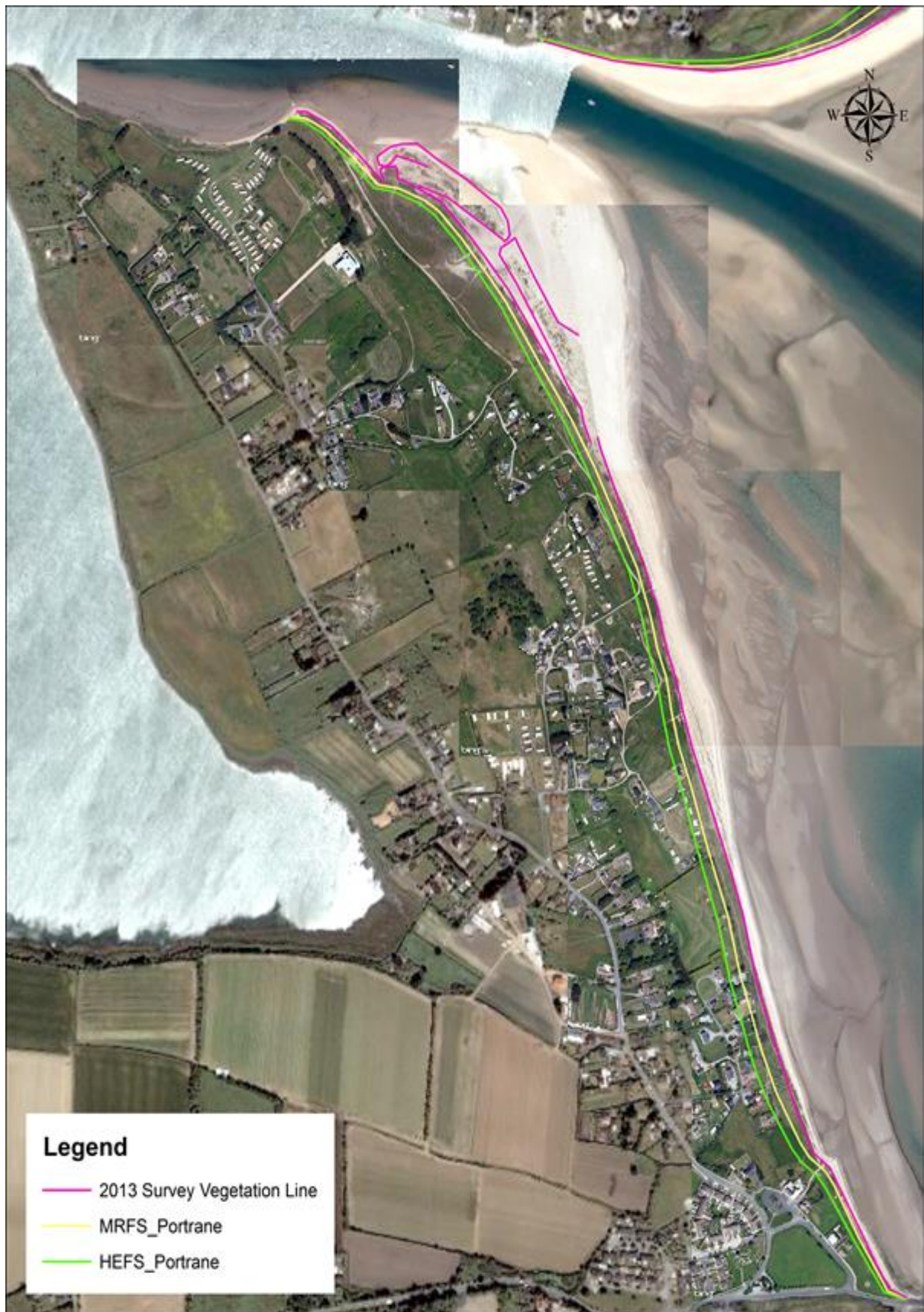
Figure 2.2: Position of the 2013 vegetation line and the 2100 MRFS and HEFS erosion lines.
