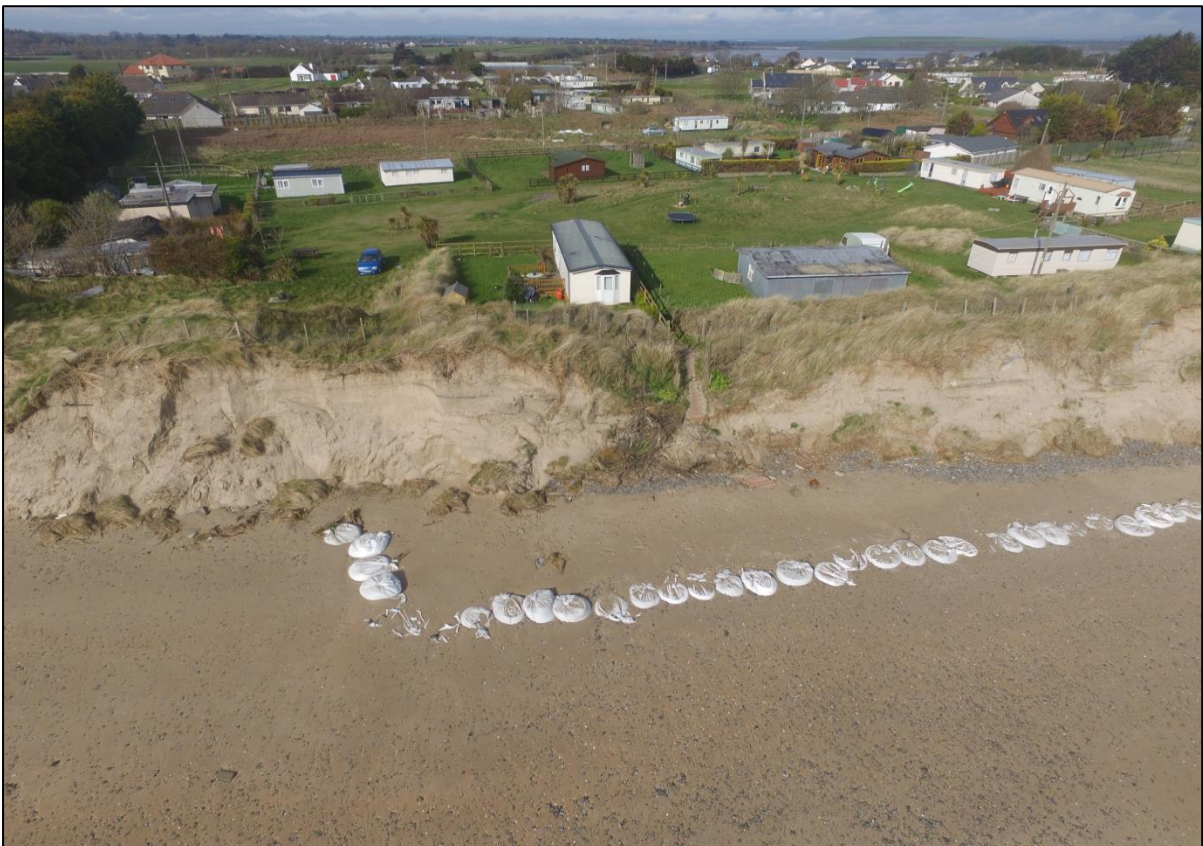
Figure 4.3: Extent and magnitude of dune erosion along the mid section of the Burrow.
