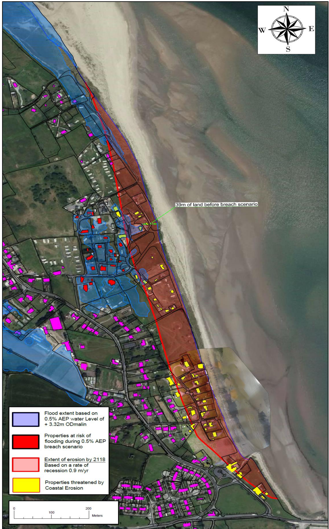
Figure 7.3: Extent of coastal erosion along the Burrow and properties at risk from erosion and flooding under a 0.5% AEP flood/breach event by 2118.
