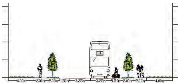
Typical Cross Section of Fosterstown link Road
