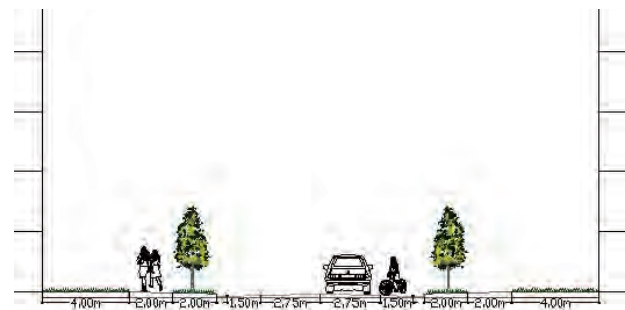
Typical Cross Section of North-South Spine Road
