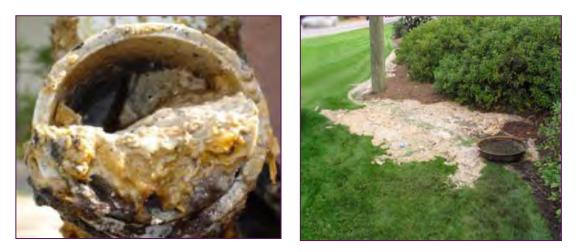
*Photographs 1 and 2 show overflows caused from FOG blockages in the sewer.*
