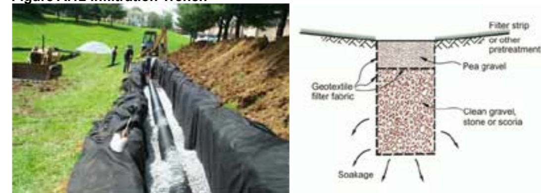
Figure A.12 Infiltration Trench
